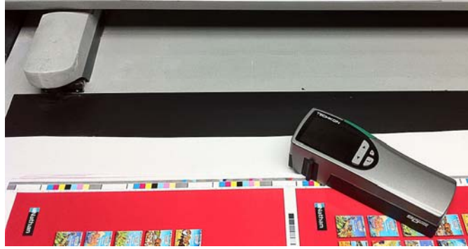
Figure 3. Techkon scanning and hand-held Spectro-Dens
