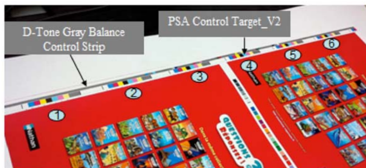
Figure 2. Print form including print job and color control bars
